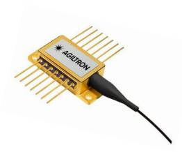
The 450nm series laser diodes are fabricated in a hermetically sealed 14-pin butterfly package. The laser diodes contain a thermoelectric cooler (TEC), and a thermistor to secure high-quality laser performance. The Laser Diodes Wavelength of 450±10nm, Output power: ≥20mW, Pigtail Type: 405-HP(Nufern) fiber with 900um loose tube, 1.0+/-0.1m, FC/APC connector. Our laser products are Telcordia GR-468 qualified and in compliance with RoHS Directives.
